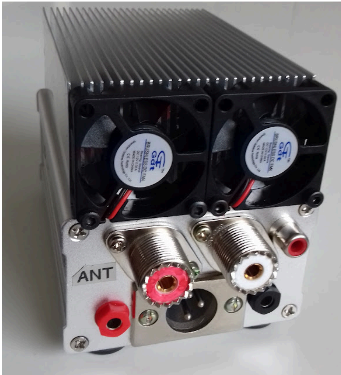
35mm cooling fans installed with LM-317 speed controll.
