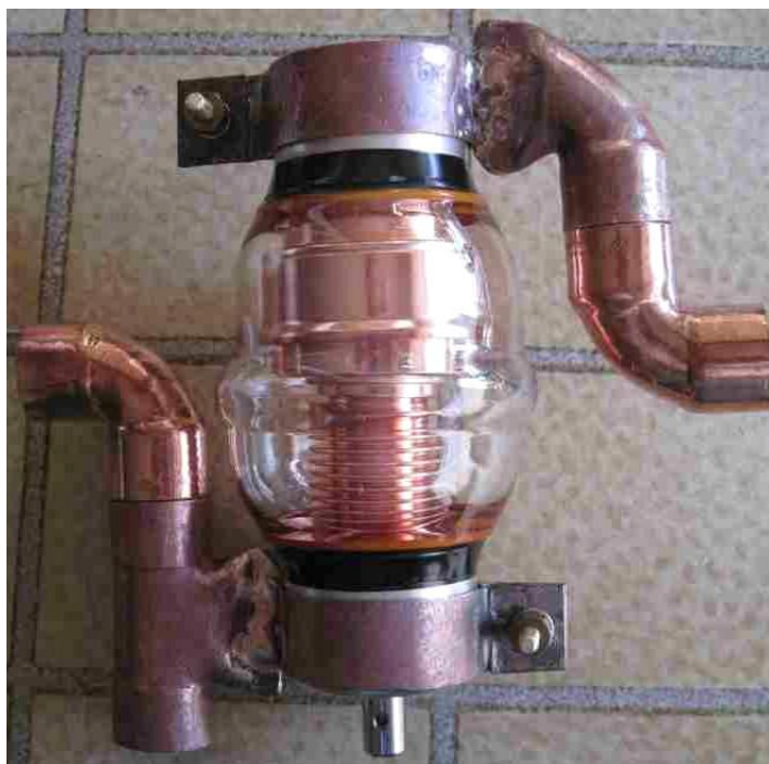
Figure 13 Homebrew capacitor clamps with silver-soldered copper fittings
