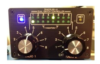
The single controller comes in two versions. The standard unit is half of a dual controller. The "Integrated" switch controller includes a band decoder that provides control of the 8-pak and FilterMax compatibly bandpass filter. Note: the Integrated Switch Controller does not include the capability to sink or source to other devices.
